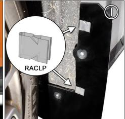
**REAR MUD FLAP** Do not fully tighten fasteners until mud flap is completely aligned to vehicle.
