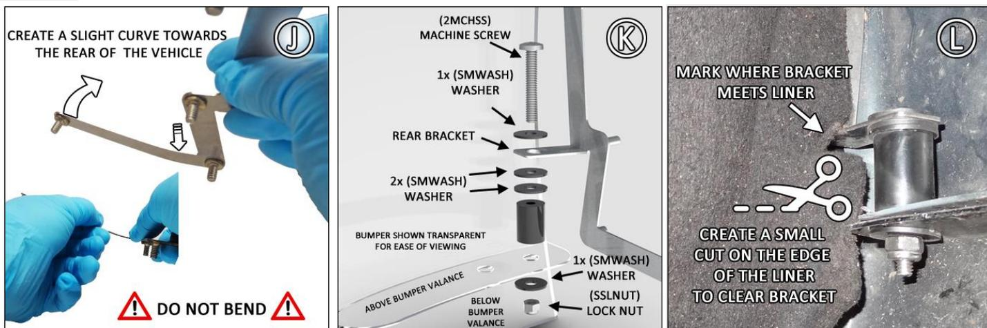
**FIGURE M** The upper portion of the bracket installs between bumper and liner. The lower bracket area requires adjustment by carefully curving the lower mount forward then backward until it seats and nests flap properly. Avoid overextending the bend.
