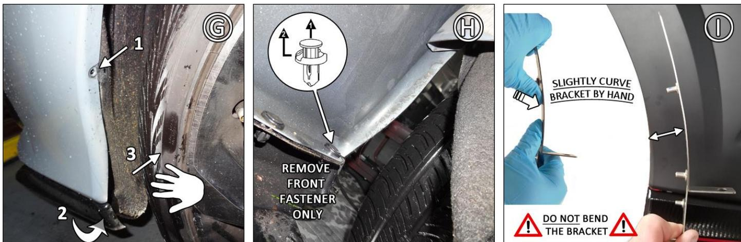
**FIGURE J** As shown in J, gently create a curve by pressing the bracket's innermost rear section close to the liner after it's installed. Do this gradually so you don't extend the curve beyond the liner. The intent is to fill the gap by bringing the part close to the liner.
