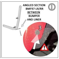
**FIGURE J** Place logo-side of flap facing rear bumper, against mounting points. Install SMWASH & factory screws into mounts 1 & 2 and SMWASH & SSLNUT into mounts 4 & 5.
