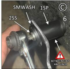
FIGURE D/E Install SMWASH & factory screws into mounts 2, 3 & 5 and INS5 into mounts 1 & 4.
