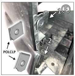
**FIGURE G** Reinstall factory fastener 3. Wipe area clean before adhering SMF103-LR/RR against mounting points. **FIGURE H** Place flap with logo facing rear bumper. Position BMF103 against flap, then install SMWASH & 1.5SS through mounts 1 & 2. Install SMWASH & HXBLT through flap and bracket mount 4. Secure with SMWASH & BLKNUT. **FIGURE I** Align mud flaps to even ground before tightening fasteners until washers are just seated.
