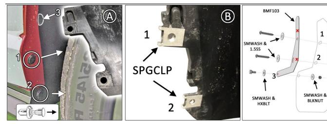
**REAR MUD FLAP** Do not fully tighten fasteners until mud flap is completely aligned to vehicle.
