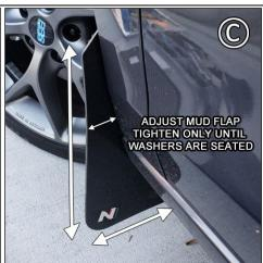
REAR FLAP Bracket/Hardware 1 x Flap →1 x BMF92-LR/RR; 3 x 1SS; 1 x INS5; 3 x SMF29-1; 5 x SMWASH; 2 x SSLNUT
