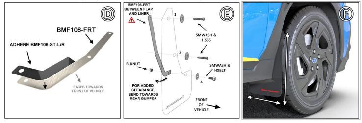
**REAR FLAP** Do not fully tighten fasteners until mud flap is completely aligned to vehicle.
