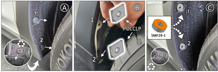
**FIGURE D/E** Place BMF106-FRT on logo-side of flap, then adhere BMF106-ST-L/R to BMF106-FRT side facing rear bumper. Install SMWASH & 1.5SS through mounts 1 & 2 and SMWASH & HXBLT through flap/bracket mount 4. Secure with BLKNUT.
