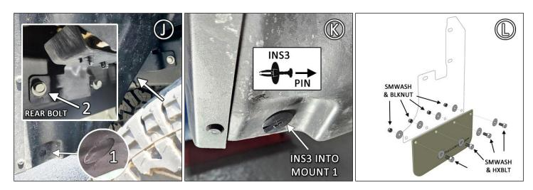
**FIGURE M** Prepare BMF84-LR2/RR2 by placing HXBLT through bracket mounts 3 – 5. HXBLT stems will point towards tire and angled tabs on bracket will face liner/rear bumper when installed.
