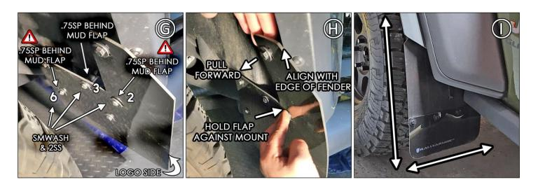
**REAR FLAP** Tighten fasteners just enough to allow for adjustment later. Bracket/Hardware 1 x FLAP → 1 x BMF84-LR2/RR2
