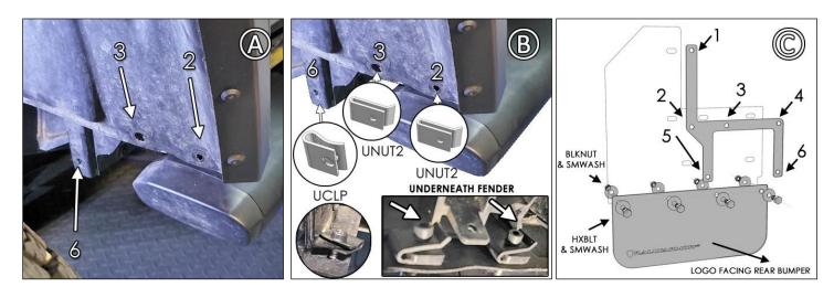
**FIGURE D/E** On tire side of flap, install SMWASH & HXBLT into BMF54-FRT mounts 1, 4 & 5. Secure logo side of flap with BLKNUT. **FIGURE F/G** Place .75SP between bracket and fender liner mounts 2, 3 & 6, then secure flap on tire side with SMWASH & 2SS.
