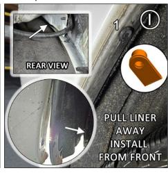
**FIGURE J** Place logo-side of flap facing rear bumper. On tire side of vehicle, place flap mount 6 UNDER liner/BEHIND factory bracket and 1SP between flap & bracket mount 6. Install SMWASH & 2MCHSS on tire side mount 6 and SMWASH & SSLNUT on reverse side.
