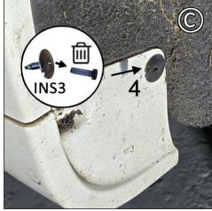
**FIGURE D/E** Place logo-side of flap facing rear bumper. Install SMWASH & 1.5SS#8 into mount 1 & .25SP <u>on its reverse</u> <u>side</u>. Adhere SMF29-1 onto .75SP. Install SMWASH & 1.5SS#8 into mount 2 & SMF29-1 /.75SP <u>on its reverse side</u>. Install SMWASH & 2.5SS#8 into mount 3 & <u>1SP on its reverse side</u>. Install SMWASH & 1.5SS#8 into mount 4 & .25SP <u>on its</u> reverse side.
