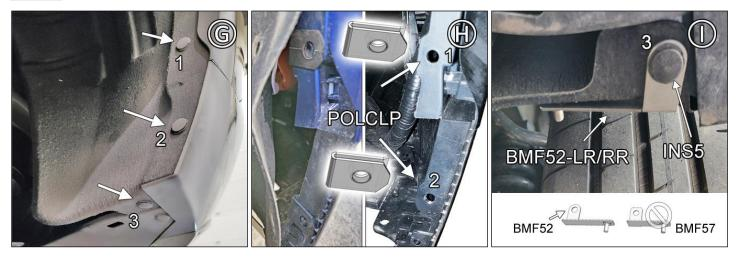
**FIGURE J** Wipe liner before adhering SMF29-1 over liner mounts 1 & 2.
