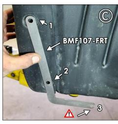
FIGURE D Install SMWASH & 1SS through mounts 1 & 2.
