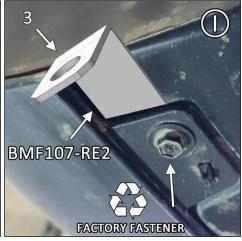
**FIGURE J** Place logo-side of flap against rear bumper. Secure mount 1 with SMWASH & 1SS and BMF107-RE & flap mount 2 with SMWASH & 1SS.
