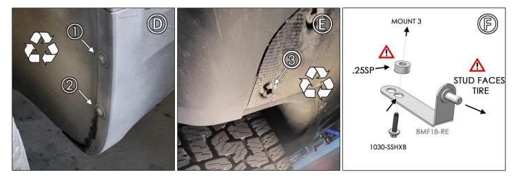
**FIGURE H** Logo-side of flap facing rear bumper, install factory fastener and WASH into mount 1. Place BMF108-RE against flap mounts, then install factory fastener into mount 2. Fasten SMWASH & SSLNUT onto mount 3. **FIGURE I** Ensure mud flap is parallel to even ground before tightening hardware just flush against flap.
