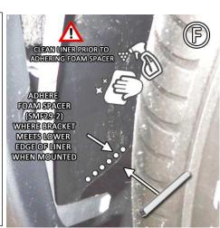
FIGURE G Referring to the arrowed mounting points in Figure G, make sure both bumper mounts line up with the 2 middle mounts on the bracket.
