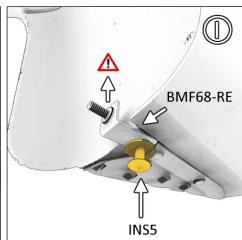
**FIGURE J** Wipe area clean. Remove SMF135-1/2 adhesive film. Attach onto liner, over mounts 1 & 2 and behind BMF68-RE stud.
