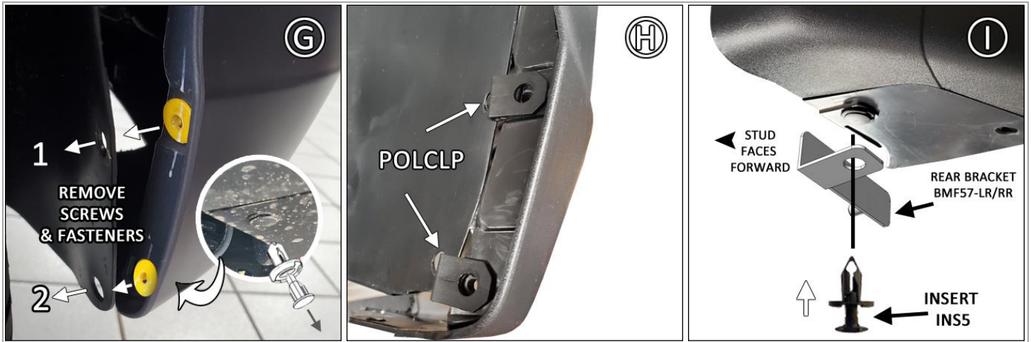
FIGURE J When mounting mud flap, .25SP Spacers mount behind mud flap against mounting points 1 and 2 as shown.
