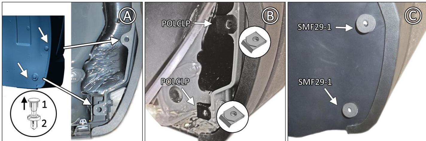
**FIGURE D/E** Place logo-side of mud flap facing rear of the vehicle against mounting points on liner. Position BMF78-FRT bracket OVER mud flap. Use WASHER SMWASH & SCREW 1SS to fasten points 1 & 2. Use a SMWASH & HXBLT and BLKNUT & SMWASH BEHIND mud flap for lower mounting point #3.
