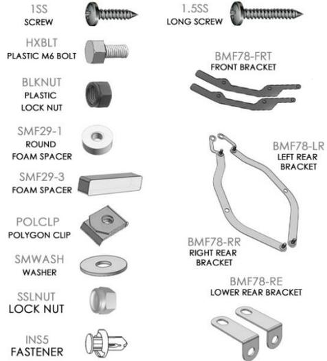
**Recommended Tools** Low-profile offset or ratcheting screw driver, 7/16<sup>th</sup> wrench, flathead screwdriver.
