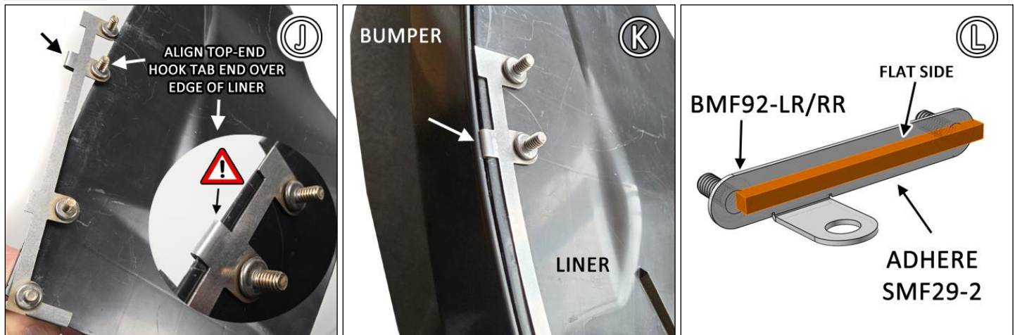
FIGURE N Fold EXPANCH, then install through BMF92-LR/RR & mount 6. Expand EXPANCH stem before fastening SMWASH & 1SS#8.
