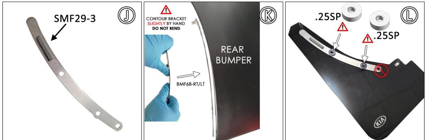
**FIGURE M** Place logo-side of mud flap facing the rear of the vehicle against corresponding mounting points of bumper. Install original screws & SMWASH through mounting points 1 & 2.
