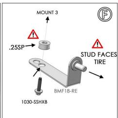
**FIGURE G** Position flap with logo facing vehicle rear against liner mounts. Loosely install factory fasteners into mounts 1 & 2. Use SMWASH and SSLNUT to secure mount 3.
